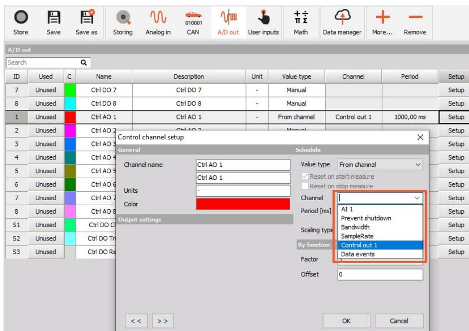
Image 25: A/D out setup, adding user input as a channel.
