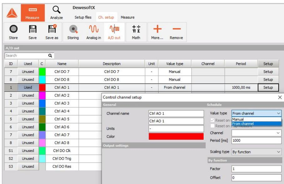
Image 5: Choosing a value type in Analog Output channel setup.
