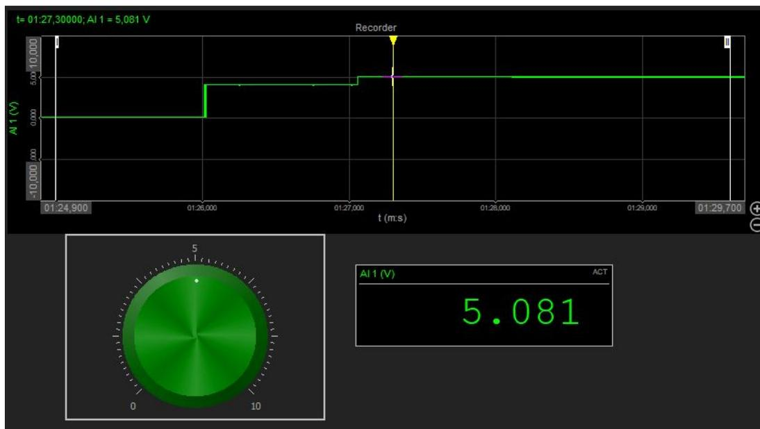
Image 26:Controlling analog output with user input.
