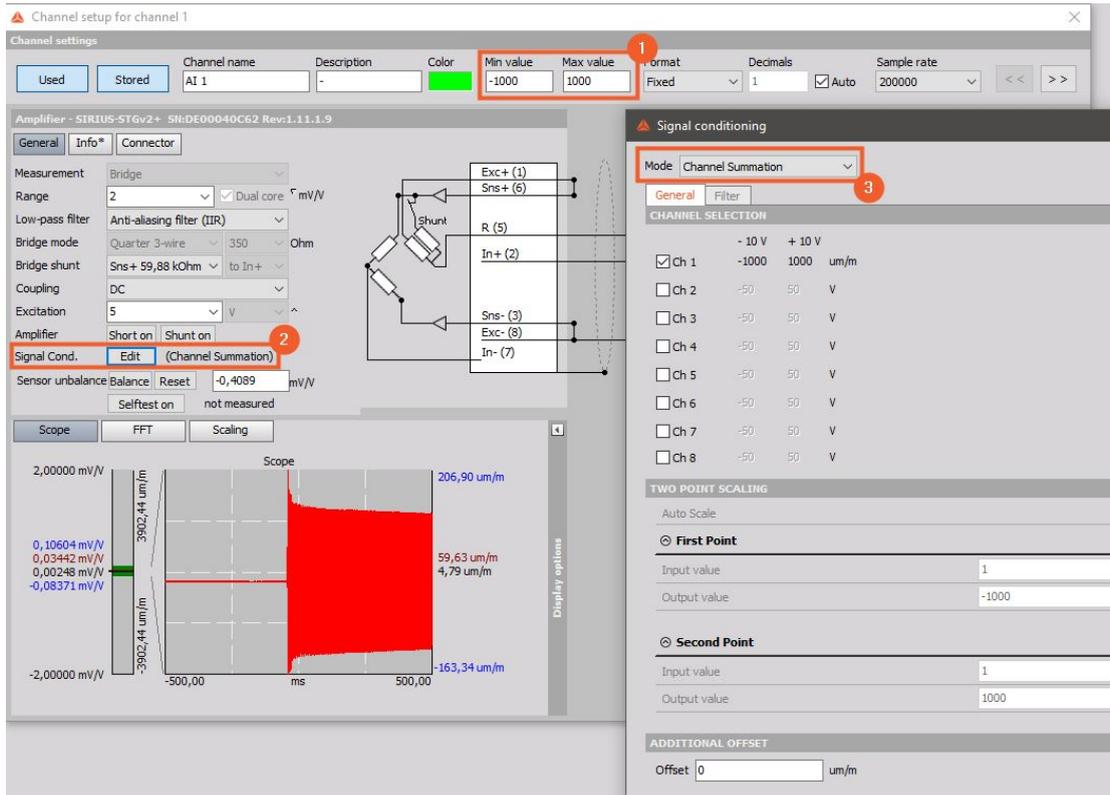
Image 6: Signal Conditioning setup at Analog Input channel setup.
