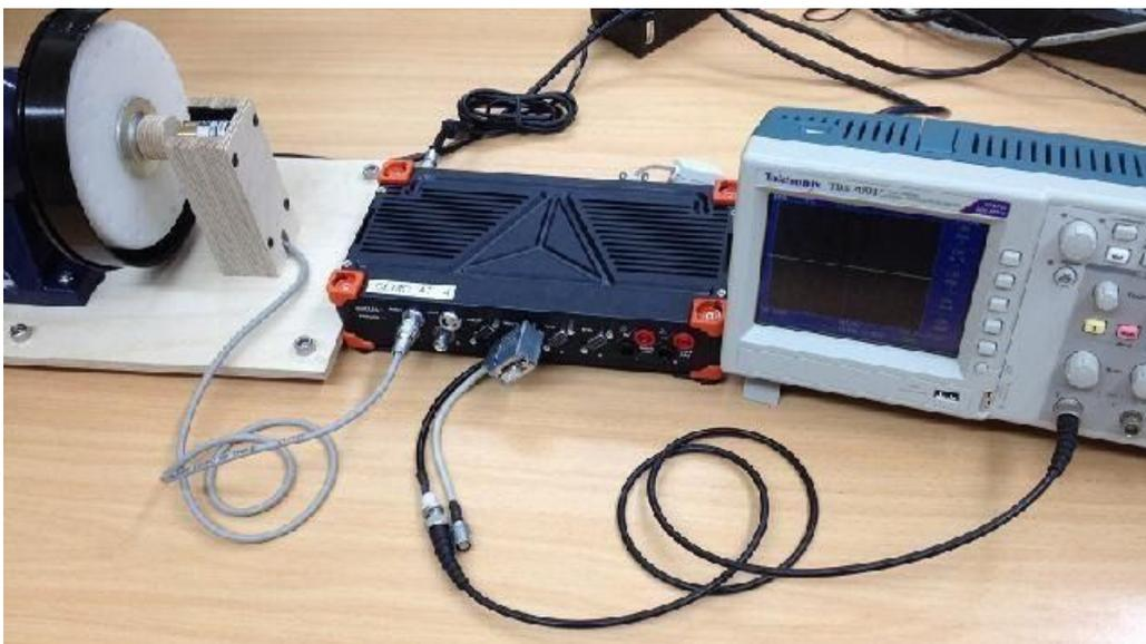
Image 36: Encoder on left and scope on right connected to SIRIUS®.
