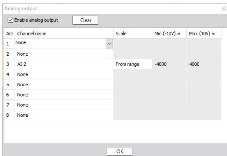
Image 16 : Analog output scale from range.
