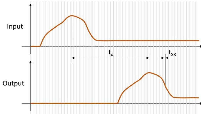
Image 35: Fast signals response rate delay.
