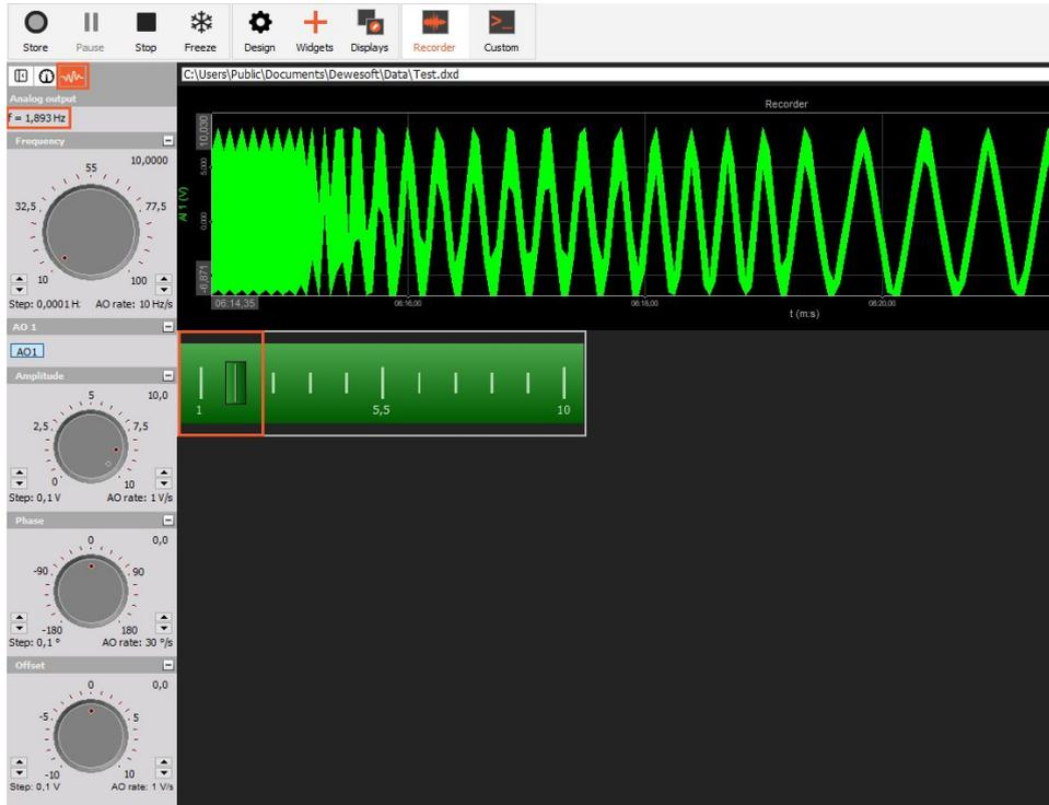
Image 32: Controlling the signal from predefined knobs or control input gadget.
