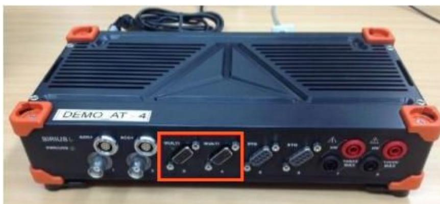
Image 14: SIRIUSi® DAQ with multi ports marked.
