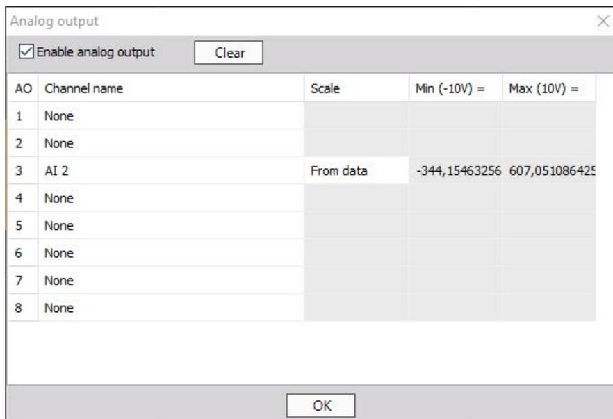
Image 18: Analog output scale from data.
