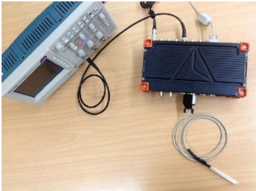
Image 22: AO on the back side of SIRIUS® connected on the oscilloscope.
