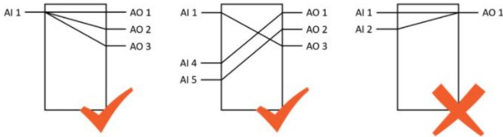
Image 23: Multiple Analog inputs can't be used for a single Analog Output.
