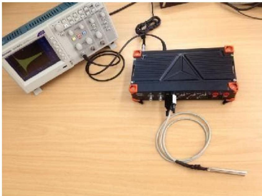
Image 9: Test setup with oscilloscope connected on rear side AO (USB not connected).
